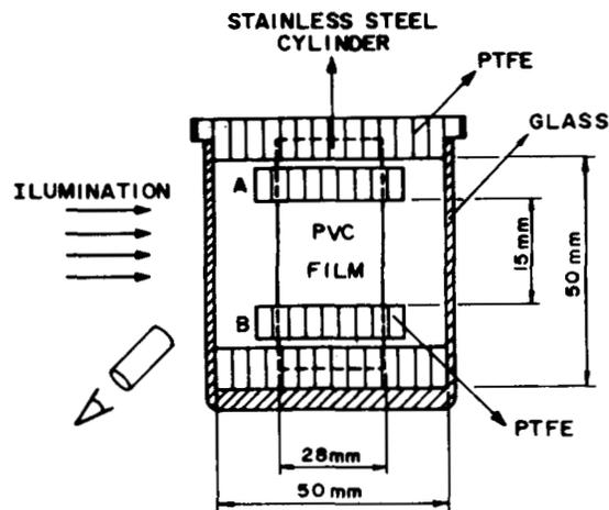
**Figure 3** Schematic diagram of the test cell. A and B indicate the removable PTFE clamps which cover the PVC film top and bottom edges.
