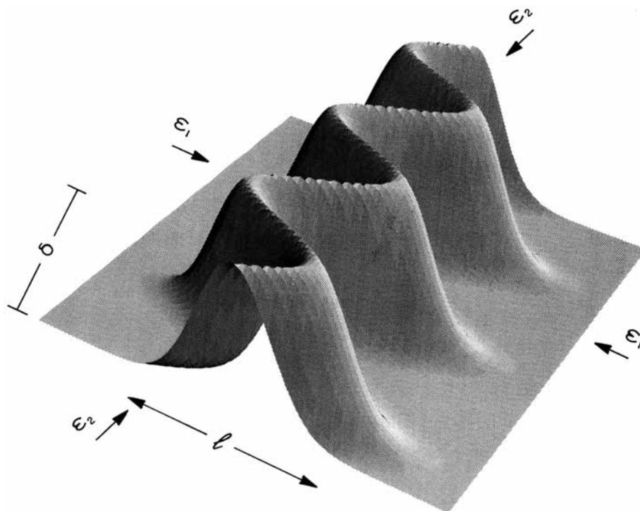
**Figure 1** Schematic representation of a wrinkled film corresponding to a tangential compressive strain  $\epsilon_1$  and axial compressive strain  $\epsilon_2$ .
