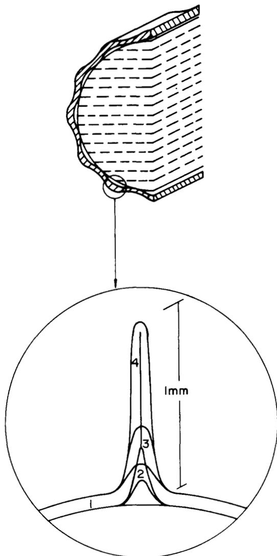
**Figure 2** Schematic diagram showing the time evolution of the striae heights. (1), (2), (3), and (4) indicate patterns formed for successively increasing times.
