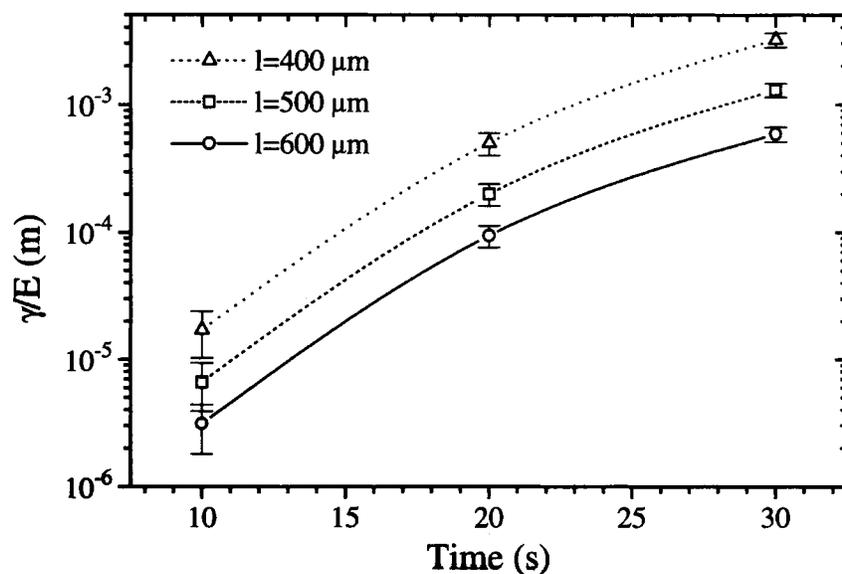
Figure 8  $\gamma/E$  dependence on the swelling time.
