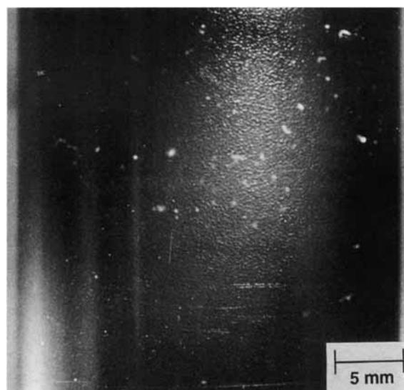
**Figure 4** Optical micrograph showing a PVC film on a stainless steel cylindrical substrate. No pattern is observed, other than normal rugosity.
